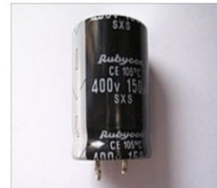
An Electrolytic Capacitor
