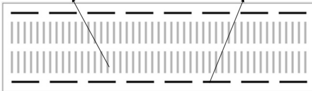
Internal Wiring Diagram of a Breadboard
