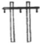
115 kV Wood H-Frame Average height 65' Average span 750'
