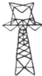
500 kV Lattice Average height 125' Average span 1150'
