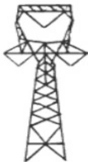
500 kV Lattice Average height 135' Average span 1150'
