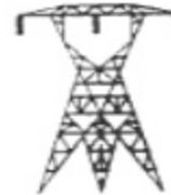
115 kV Steel Lattice Average height 75' Average span 1150'
