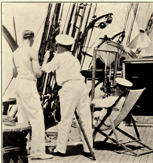
FIGURE 5.—Observing the course of a pilot balloon with theodolite and sextant. The spring supporting the sextant hangs from a screw eye in the bar over the chair
