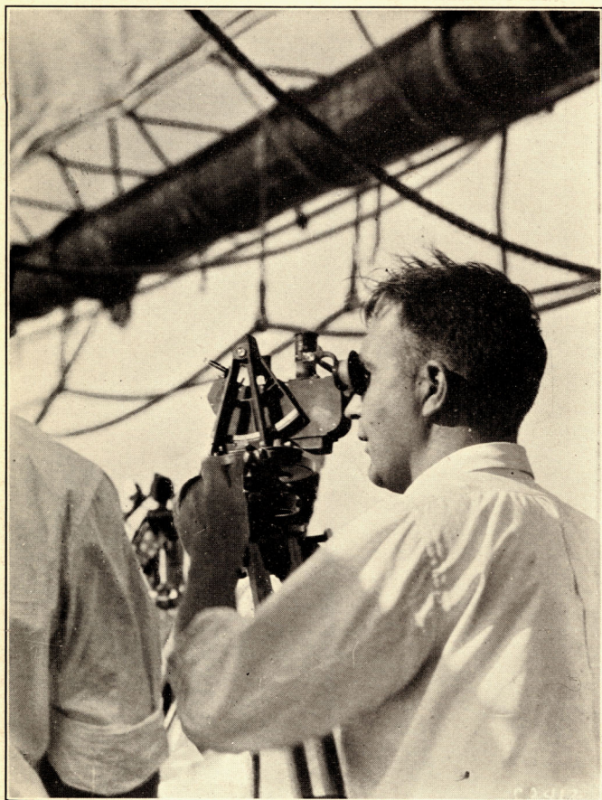
FIGURE 4.—Observing the course of a pilot balloon with the United States Navy theodolite
