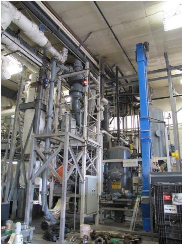
Figure 3.1 Bubbling fluidized bed gasifier
