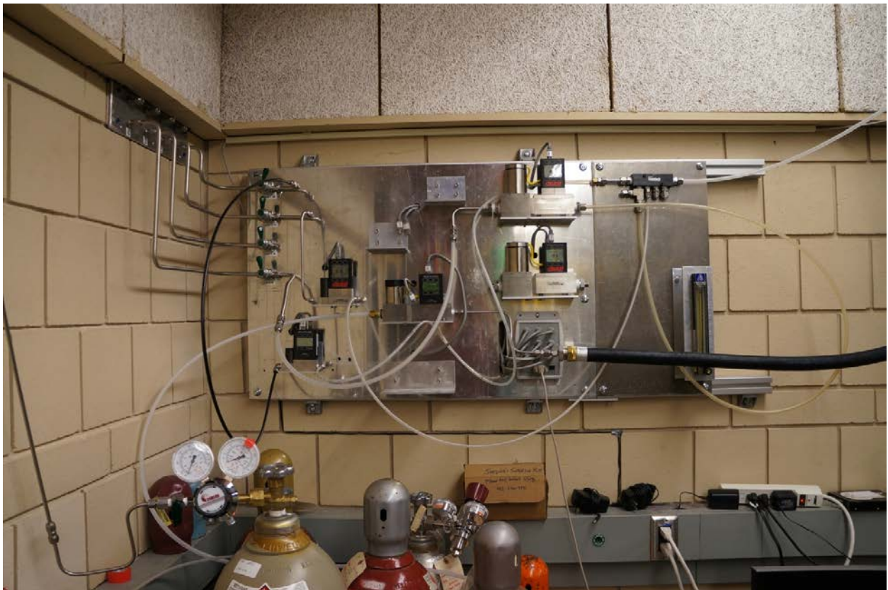
Figure 4.3 Mass flow controller setup
