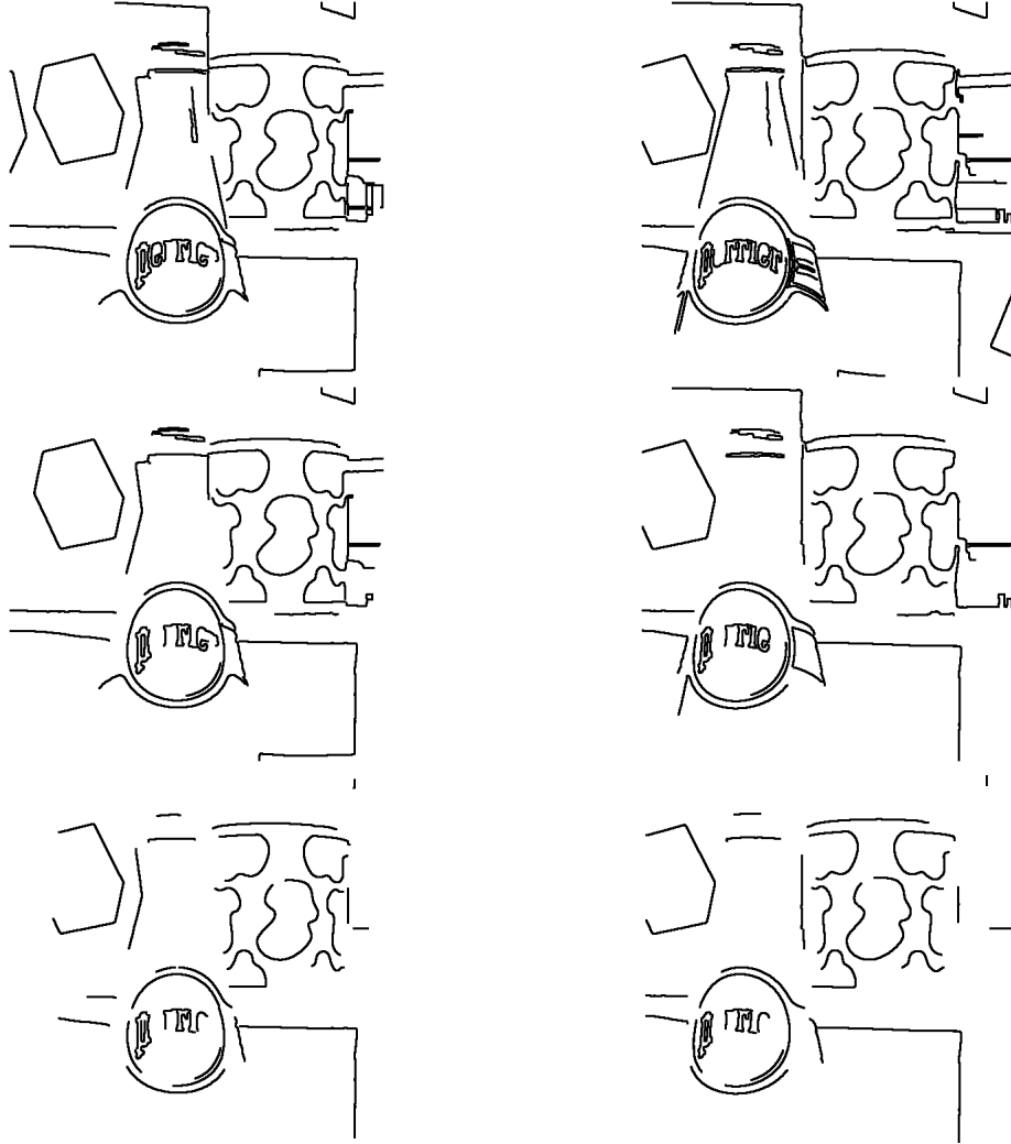
Fig. 5. Short baseline matching. Upper pair : Contours extracted with CannyOx (parameters: min grad 60, min length 60). 37 and 47 contours are obtained for the left and right images respectively; Middle pair : Contours which are matched between views. Lower pair : Matched contours showing only the parts which have corresponding edgels in both views. 97% of the 29 matches are correct.
