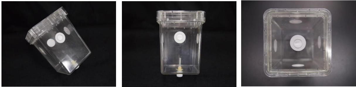
Fig. 2.1 Photos of the Plant Chamber with air ventilation holes covered in gas-permeable membrane.
