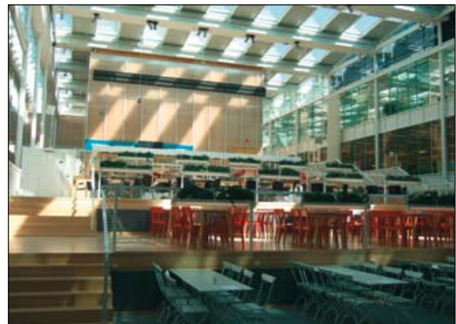
Figure 3. The electric and natural light in the atrium can be adjusted as required via remote control.
