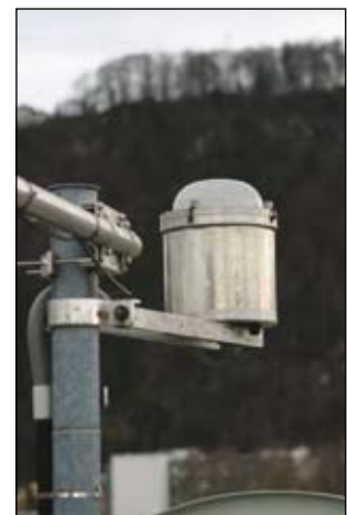
Figure 2. The heated measurement container with the light value sensors.
