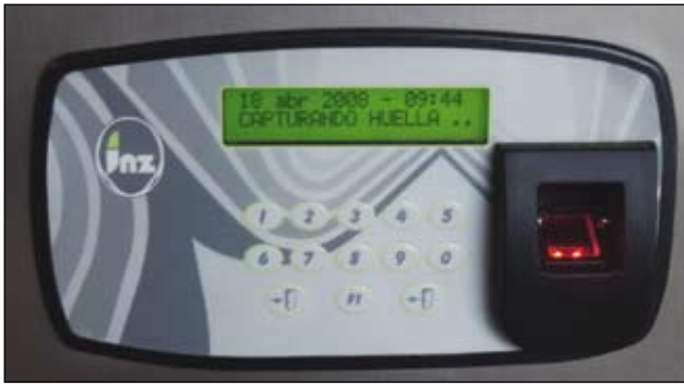
Picture 4. Thanks to the interface of the access control system (fingerprint) to the KNX system, a customized control of all systems is possible.
