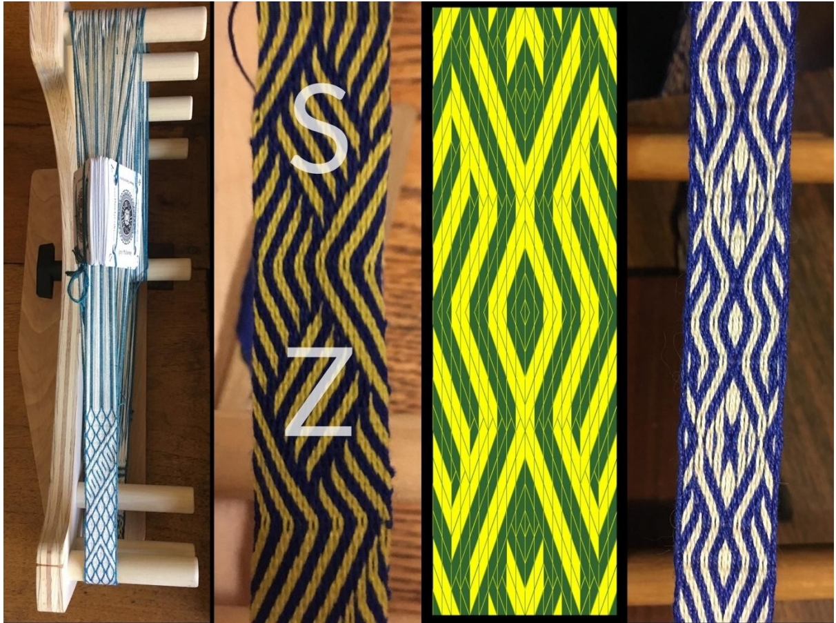
Figure 5: The figure shows (from left to right): The process of tablet weaving with a woven piece on the bottom and the twistable tablets between the strings, a distinction between the S and Z direction, a computer model of the weaving process, and its physical realisation.
