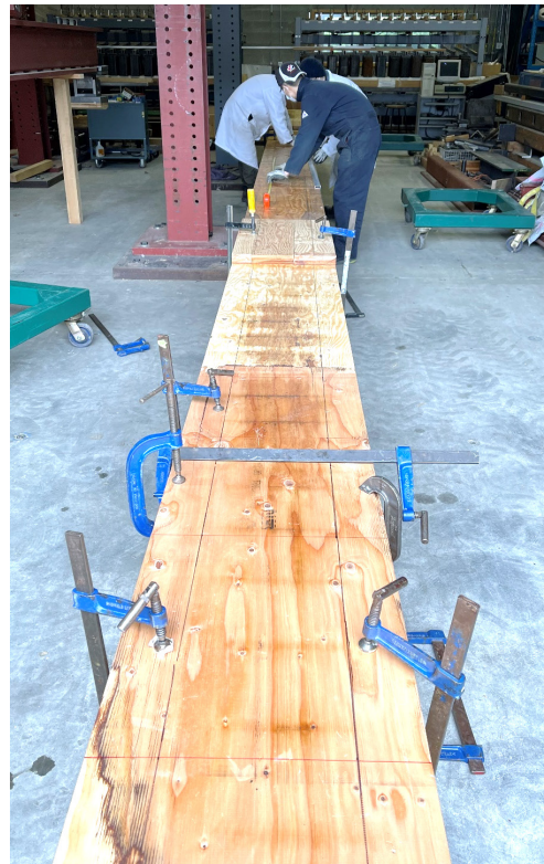
Figure 4 Configuration and manufacturing of the composite floor
