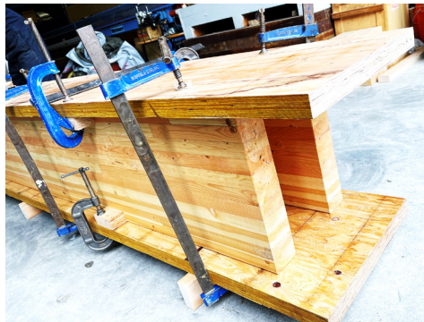
Figure 4 Configuration and manufacturing of the composite floor
