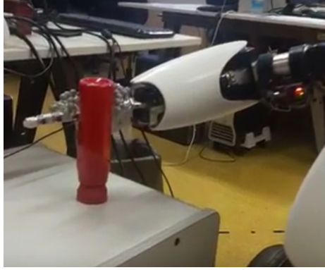
Fig. 1: Example of the initial robot configuration before the execution of a precision grip experiment for weight estimation
