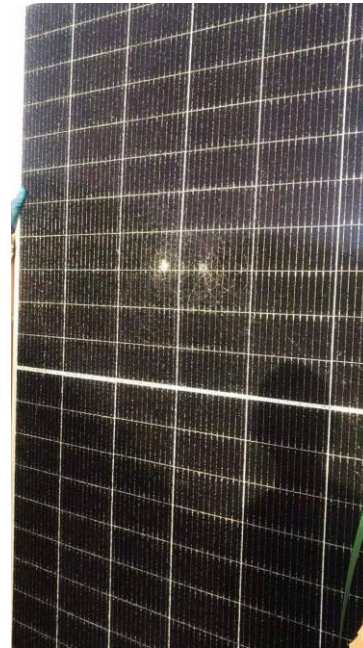
Damaged module
