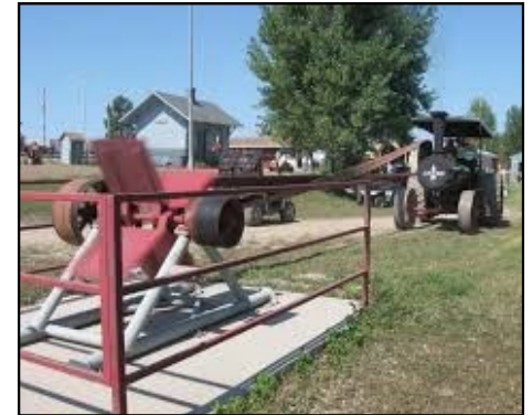
A Baker Fan at the Western Minnesota Steam Thresherman's Reunion in Rolla, MN. The fan produces the load. Horsepower is determined by the dimensions of the fan and RPMs but is sensitive to air density (temperature, barometric pressure, humidity, and elevation).
