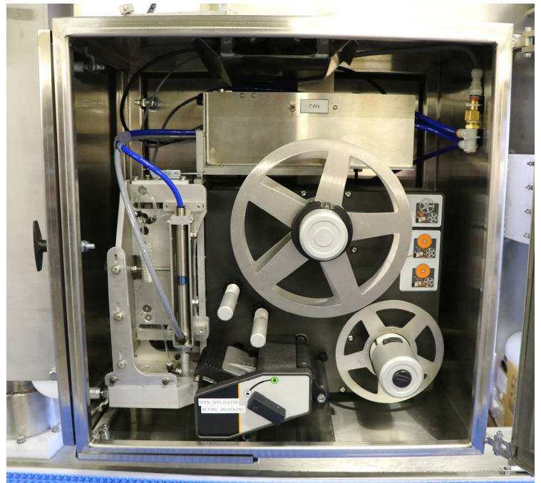
The majority of our weigh price labeling systems are outfitted with an applicator that applies labels with high speed and precision to the base and/or top of packages.
