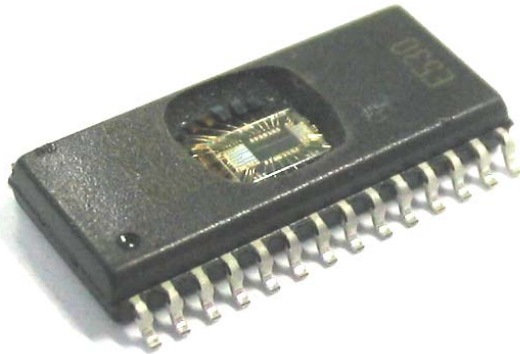
Figure 8 View on the test device. The test chip is encapsulated in the plastic package P-DSO-28 (molding compound partially removed above the test chip) [11]
